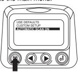
Touch the "Menu Button" to exit the Main menu and return to the engine parameter display.
